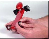
5. Roll test the car on a smooth, horizontal surface. The car should roll freely, and the wheels should spin without restriction. Make adjustments if necessary.
